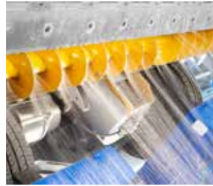
Screw conveyor wash system horizontal can be activated during ice resurfacing
