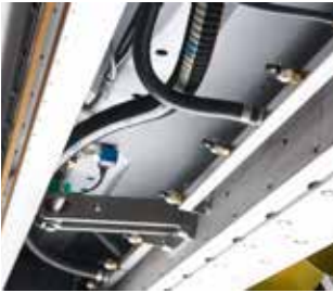
Ice wash system Multijet with suction ledge
