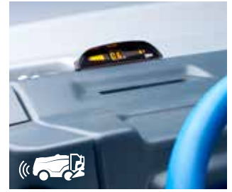
Acoustic distance warning system front
