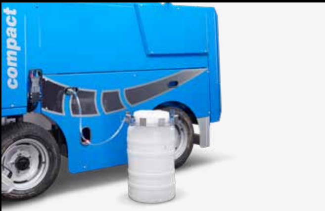
Battery watering system
