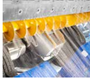
Screw conveyor wash system horizontal
