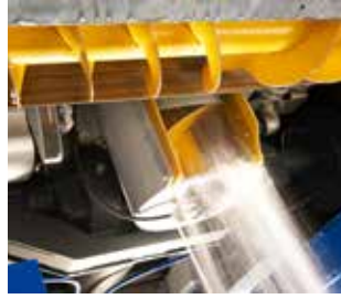
Screw conveyor wash system vertical
