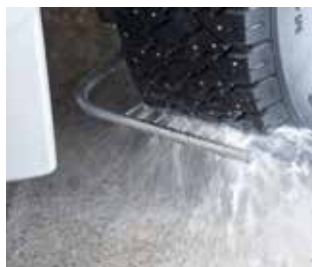
Wheel wash system with co-steering
