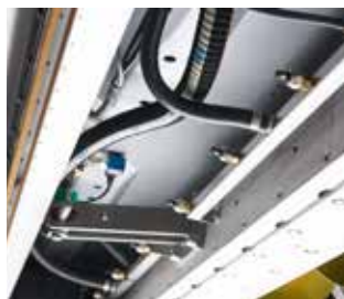
Ice wash system Multijet with suction ledge
