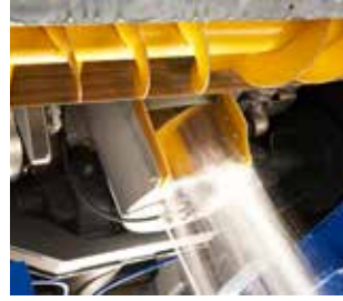
Screw conveyor wash system vertical can be activated during ice resurfacing
