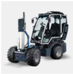
Implement mast with hydraulic block unit & additional hydraulic functions
