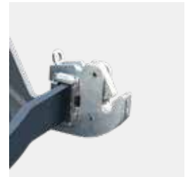
Quick-release hooks for linkage type Fendt Ø 22
