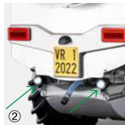
2 LED work lights for HQS
