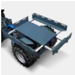
Transportation platform (adjustable in length and width)
