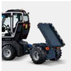
Tilting device with hydraulic actuation
