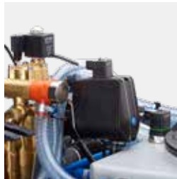
Pressure sensor and electric pressure regulator
