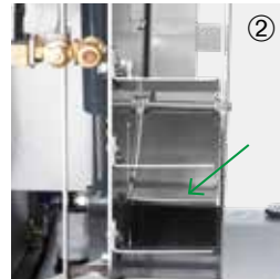
Angle sensor and hydraulically adjustable flaps for HQS
