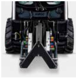
Hydraulic power unit & 12V socket
