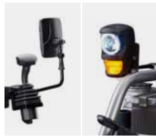
Road homologation kit (Lights, horn, rear-view mirror, registration plate, holder)
