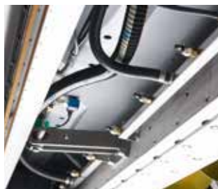
Ice wash system Multijet with suction ledge
