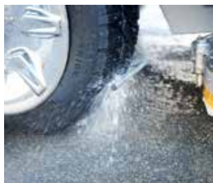
Wheel wash system with steering
