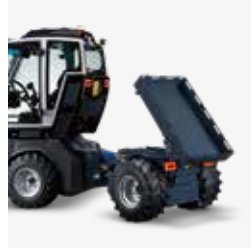
Tilting device with hydraulic actuation
