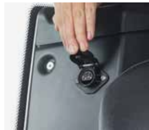
Switchable 12V socket according to DIN 9680
