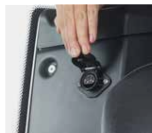
Switchable 12V socket according to DIN 9680
