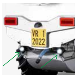
2 LED work lights for HQS
