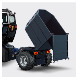
Tilting device with hydraulic actuation
