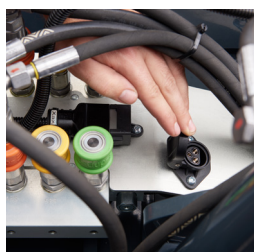
Switchable 12V socket according to DIN 9680
