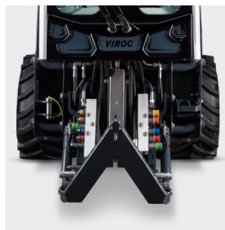
Hydraulic power unit & 12V socket
