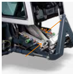
Hydraulic power unit & 12V socket
