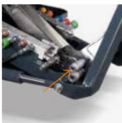
Ports for the second gear pump
