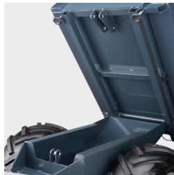
Frame with manual tilt function
