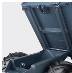
Frame with manual tilt function
